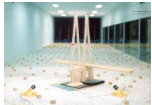
Fig. 10 Free Standing Tower Test Set-up
